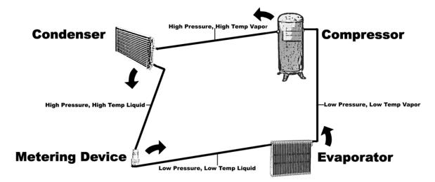
The **refrigeration process** is essentially the transfer of heat from one place to another. In an air conditioning unit, for example, the heat is removed from inside the building and is deposited outside the building. The vapor-compression refrigeration cycle is a repeating cycle consisting of four main components: evaporator, compressor, condenser and metering device.
