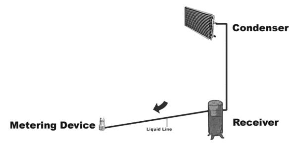
Systems using thermal expansion valves will have a receiver/tank on the outlet side of the condenser, designed to hold liquid refrigerant. When leaving the condenser directly or the receiver, the refrigerant remains a high pressure/high temperature liquid until it goes to the
